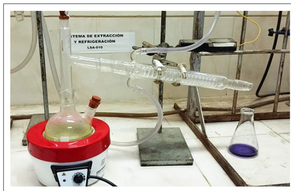
Figure 4. Working distillation equipment arrangement (IIDEPROQ)
